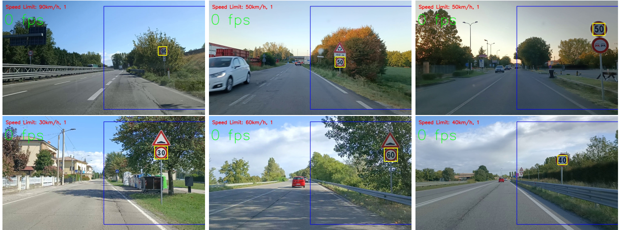
Figure 4: Traffic sign detection and classification done by our technique
