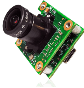
Figure 8: See3CAM_CU27 Full HD Sony R Starvis TM IMX462 Ultra Low Light USB 3.1 Gen 1 Camera
